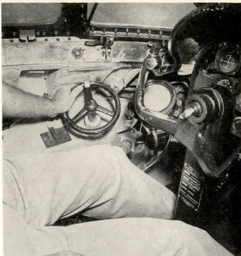
The nose steering which does not turn the nosewheels. It actuates the valve to direct hydraulic pressure to do the steering.
